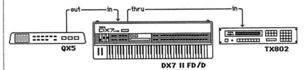
With Local Control on, the DX7 II can control both its own sounds and those of the external tone generator; the DX7's internal sounds are also being controlled by the sequencer. With Local Control off, the DX7 II controls only the external tone generator, while its internal sounds are "played" by the sequencer.
