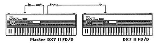
Turn Local Control "off" on the first (master) DX7 II. (Refer to Section 4 for details.)
