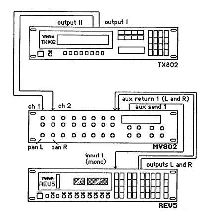
Note: The MV802 mixer in this setup may be omitted. To omit the MV802, please connect the I and II outputs of the TX802 into the REV5's inputs, then connect the REV5's outputs into your amplification system. Use the REV5's mixing control located on the front panel to balance the dry signal with the effects.
